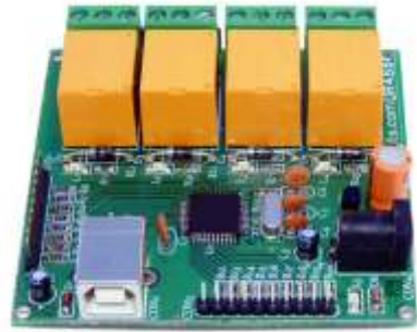
R242 is an RS232 based Relay Card having up to 9 I/O channels & 4 ADC channels. The ADC resolution is 10 bits.
