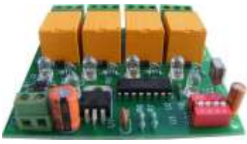
6 channel I R Remote control Board - AZ6CR-03
