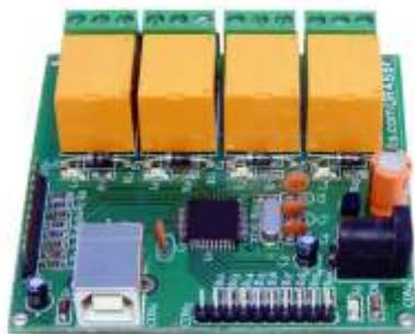
R242 is an RS232 based Relay Card having up to 9 I/O channels & 4 ADC channels. The ADC resolution is 10 bits.
