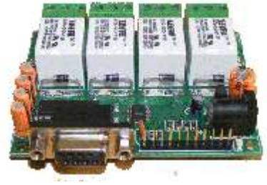
R242 is an RS232 based DAQ & Relay Card having up to 9 I/O channels including 4 ADC channels. The ADC resolution is 10 bits . There are 4 onboard relays.
