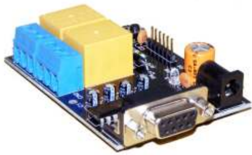
iRS-2R is an RS232 based DAQ & Relay Card having up to 4 I/O channels including 4 ADC channels. The ADC resolution is 10 bits . There are 2 onboard relays.
