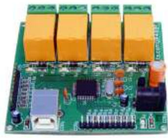
R242 is an RS232 based DAQ & Relay Card having up to 9 I/O channels including 4 ADC channels. The ADC resolution is 10 bits . There are 4 onboard relays.
