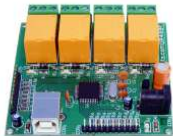
R242 is an RS232 based DAQ & Relay Card having up to 9 I/O channels including 4 ADC channels. The ADC resolution is 10 bits . There are 4 onboard relays.
