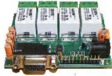
R242 is an RS232 based DAQ & Relay Card having up to 9 I/O channels including 4 ADC channels. The ADC resolution is 10 bits . There are 4 onboard relays.
