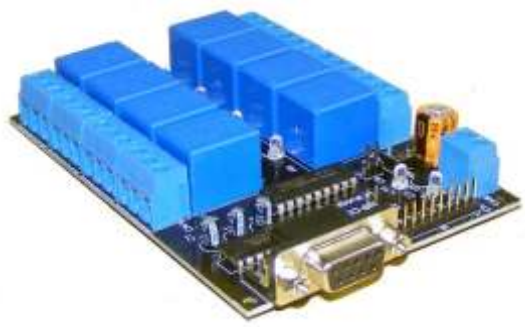
iRSD-8R is an RS232 based DAQ & Relay Card having up to 8 I/O channels including 4 ADC channels. The ADC resolution is 10 bits . There are 8 onboard relays.
