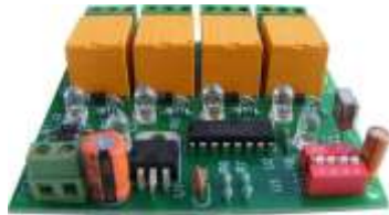
6 channel I R Remote control Board - AZ6CR-03
