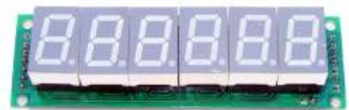
6 digit 7 segment Multipurpose LED Counter
